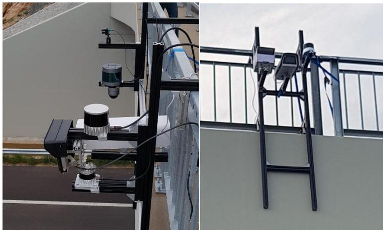
*Fig. 3 Perception sensor system at the first test session (left) and at the second test session (right)*
