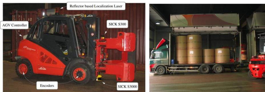
**Fig. 2** Autonomous forklift for truck loading [10]
