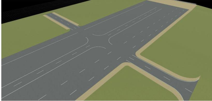
*Fig. 4 Road model of ZalaZONE ADAS surface in RoadRunner software*
